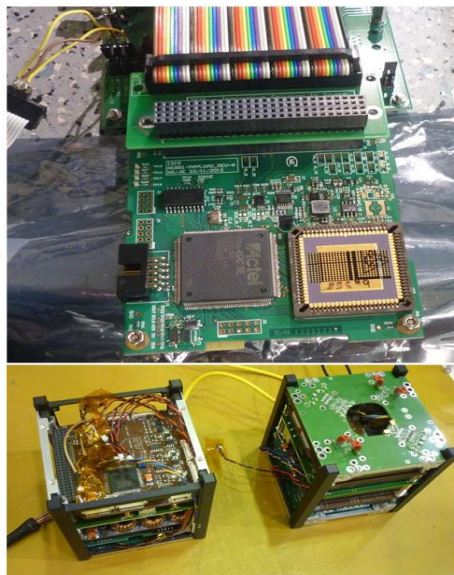
Figure 4: The NANOSATC-BR1's Payload Circuit Board and Engineering Model Platform (EM), the Flight Model Platform (FM).
