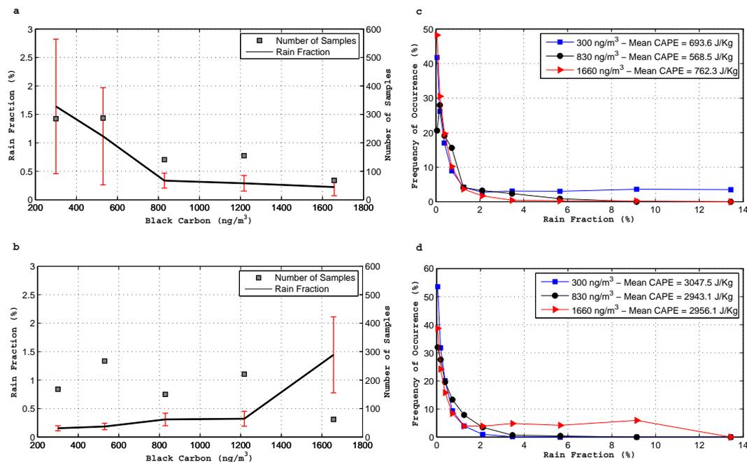
**Figure 4.** Mean, standard deviation, and number of samples of rain fraction (RF) for different black carbon (BC) concentrations for less unstable (a) and more unstable (b) atmospheres in the dry period. RF frequency histograms for the first, third, and fifth BC concentrations in (a) and (b), are shown for less unstable (c) and more unstable (d) atmospheres. The first and third curves in (c) and (d) are significantly different as determined by a *t* test at the 95 % confidence level.
