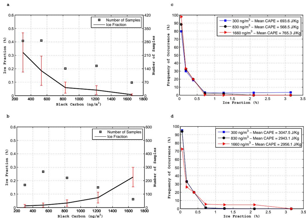
**Figure 5.** Mean, standard deviation, and number of samples of ice fraction (IF) for different black carbon (BC) concentrations for stable (a) and unstable (b) atmospheres in the dry period. IF frequency histograms for the first, third, and fifth BC concentrations in (a) and (b) are shown for less unstable (c) and more unstable (d) atmospheres. The first and third curves in (c) and (d) are significantly different as determined by a *t* test at the 95 % confidence level.
