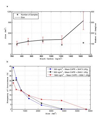
**Figure 6.** (a) Mean, standard deviation, and number of samples of rain cell size  $(>100 \, \mathrm{km^2})$  for different black carbon (BC) concentrations in a more unstable atmosphere during the dry period; (b) size frequency histograms for the first, third, and fifth BC concentrations in (a). The first and third curves in (b) are significantly different, as determined by a t test at the 95 % confidence level.
