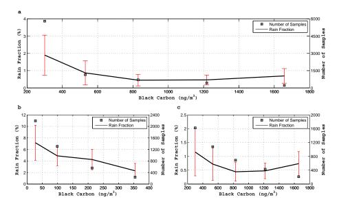
**Figure 3.** Mean, standard deviation, and number of samples of rain fraction (RF) for different black carbon (BC) concentrations. (a) Entire year; (b) rainy season; (c) dry season. For these curves, no atmospheric stability consideration was performed.
