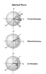
Figure 2. Spherical waves. From top to bottom are circular polarized, elliptical polarized and arc polarized waves. All three waves have constant magnetic field magnitudes. An arc polarized wave is a nonlinear extension of a small amplitude linearly polarized wave. Taken from Tsurutani and Lakhina (2000). See also Tsurutani and Ho (1999).
