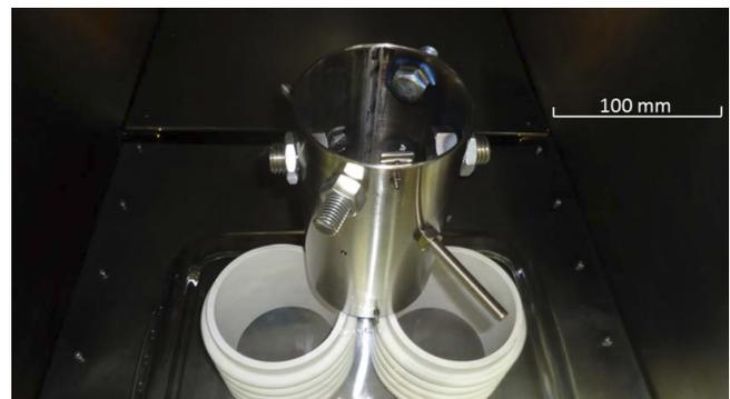
FIG. 4. Photo of the tube fixture loaded with components and samples after PIII treatments.
