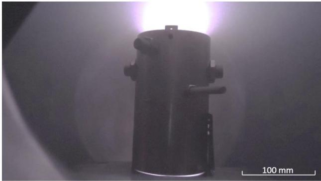
FIG. 5. Side view picture of the tube fixture loaded with industrial components during PIII treatment.
