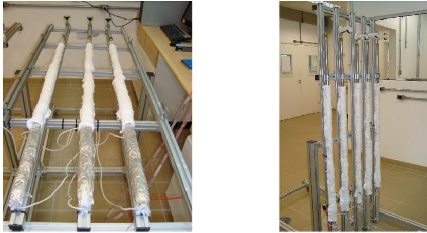
**Figure 1 - Heat pipes experimental test rig.**
