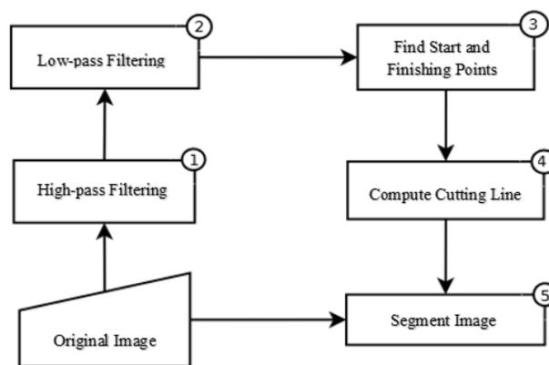
Fig. 1 - Scheme for segmenting images using tiles.
