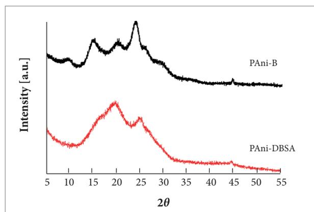
**Figure 6.** XRD pattern of PANi-B and PANi-DBSA.
