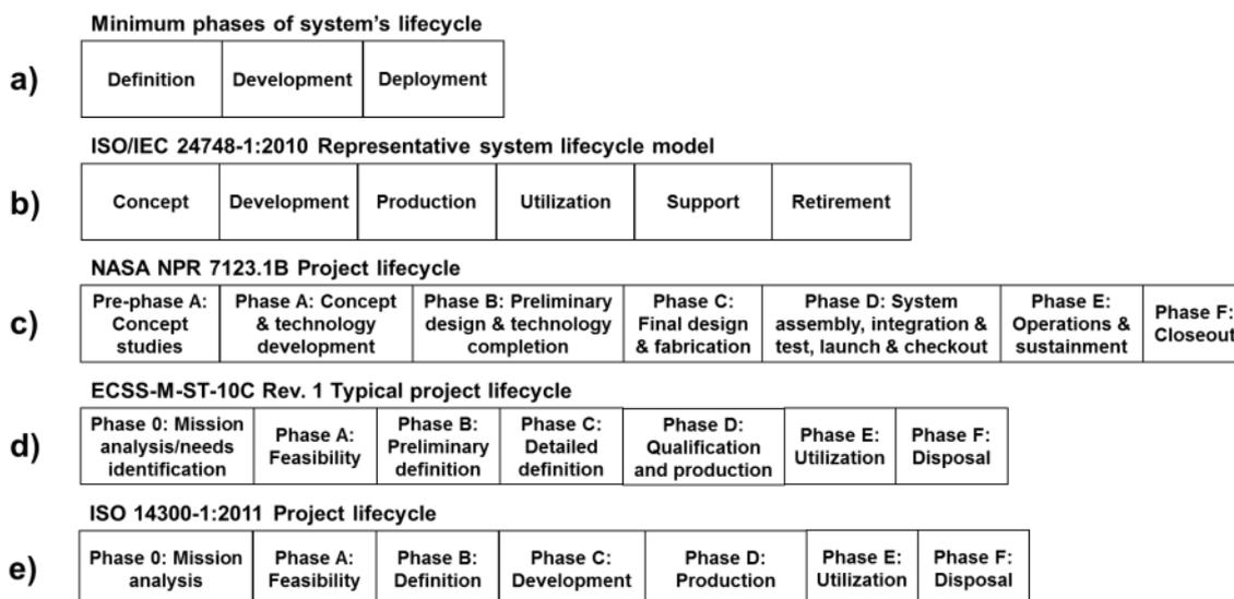
Item 'a)' shows the minimum phases that a system lifecycle must have according to Sage and Armstrong Jr. (2000). Item 'b)' shows a generic system lifecycle model according to ISO and IEC (2010). Item 'c)' shows the space project lifecycle according to NASA (2013). Item 'd)' shows the space project lifecycle according to ECSS (2009a). Finally, item 'e)' shows the space project lifecycle according to ISO (2011).
