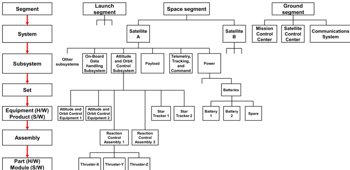
*In the left side, the figure illustrates the names of the hierarchical levels. In the right side, the figure illustrates an example of a space system decomposition.*
