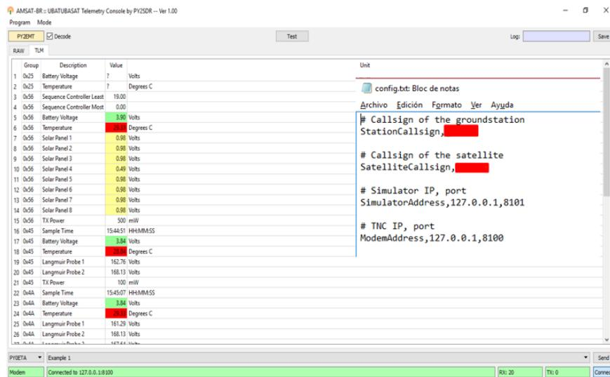
Figure 9. UbaTM Decoder with engineering valued telemetry and configuration file.
