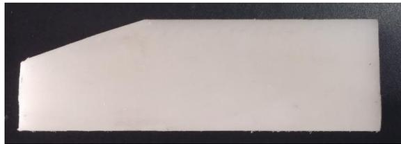
Figure 6: Chamfered HDPE grain.
