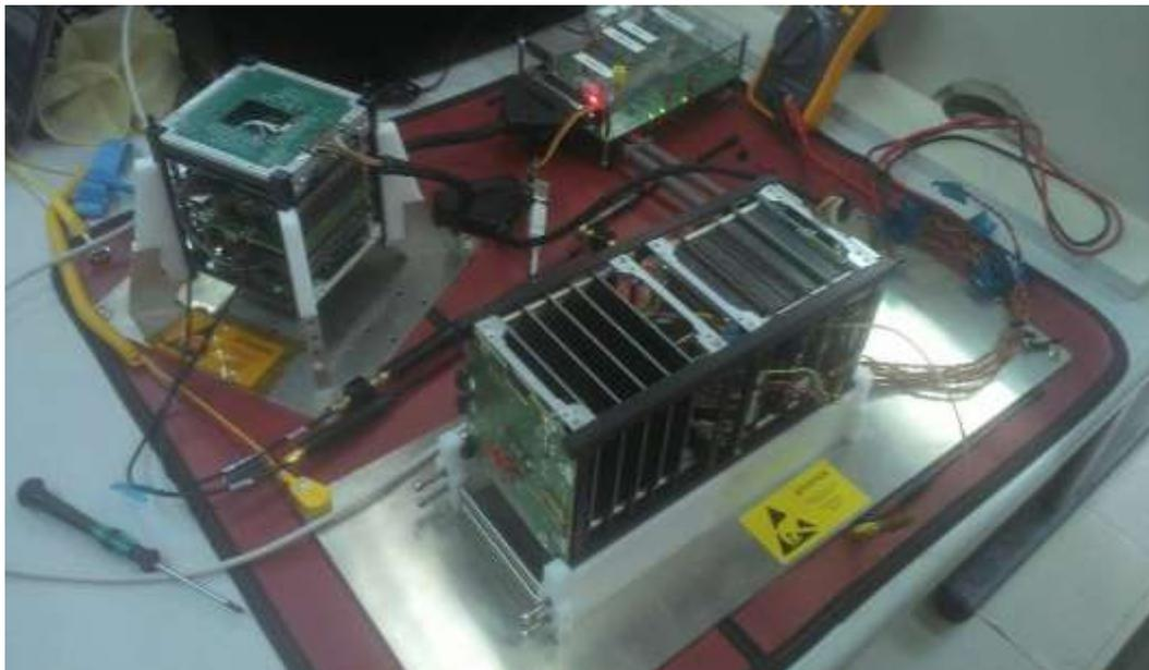
**Figure 1: The NANOSATC-BR1 and NANOSATC-BR2 Engineering Model Platforms.**
