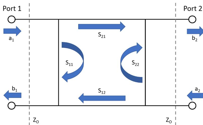
Fig.1 Schematic representation of a device with two ports [8]. The symbols a and b represent the amplitude of the incident wave and the response.
