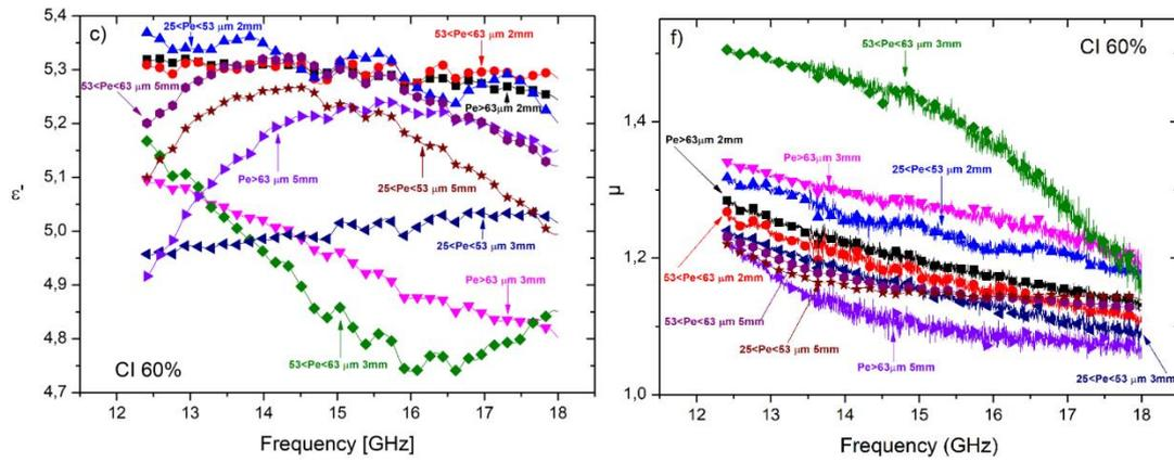
Fig.4 Experimental values of the real part of the permittivity (a) (b) and (c) and permeability (d), (e) and f) as a function of frequency.
