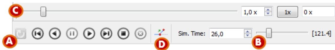
Figure 5.15 - Playback control panel: (A) execution control; (B) simulation horizon slider; (C) acceleration factor slider and edit fields; (D) scenario branch generation.
