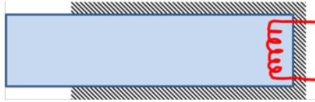
(a) The bar is  $\frac{4}{5}$  fully insulated and has a  $20W$  heater attached to one of its end.
