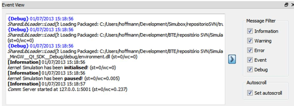
Figure 5.13 - Event viewer window used to display messages logged from simulator kernel and model.
