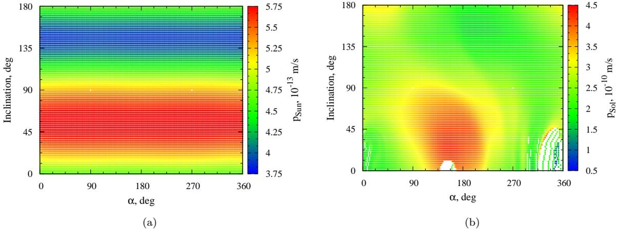
Figure 4. Total velocity contribution due to the Sun, as a function of the initial inclination and angle of approach, for  $R_p = 4RP$  (a) and  $R_p = 50RP$  (b).
