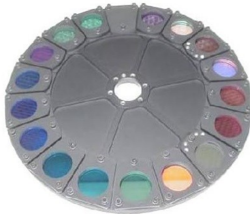
Figure 3.4 – Filter wheel of the HST WFC3 camera.
