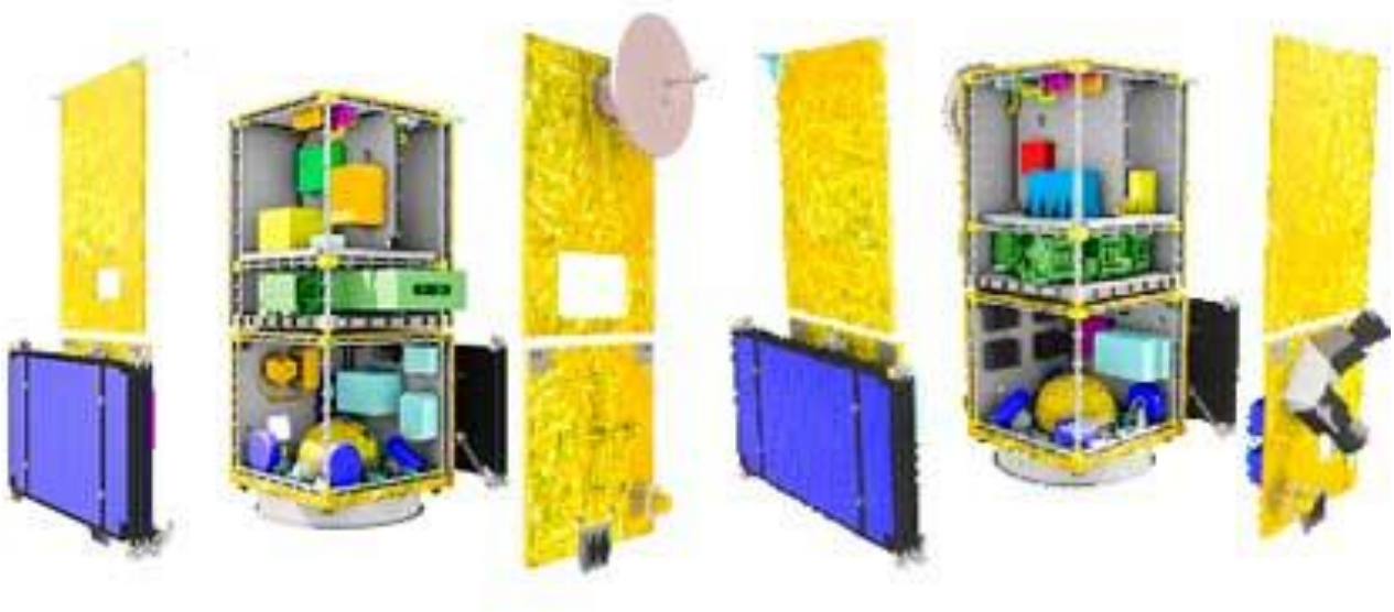
Figure 3. Amazonia-1 satellite with his two-coupled modules
