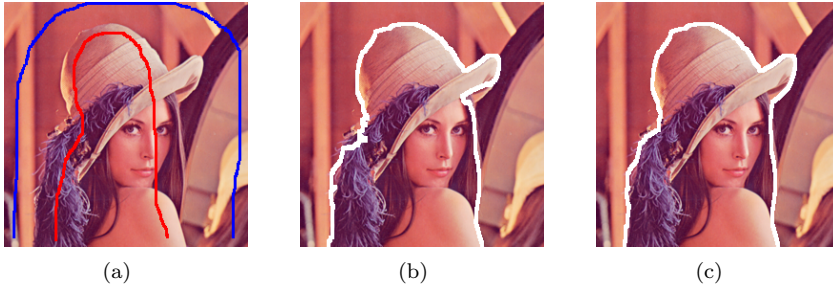
Figure 5. Color image segmentation: (a) markers superimposed to the original image; (b) watershed on P ; (c) min-cut on P .
