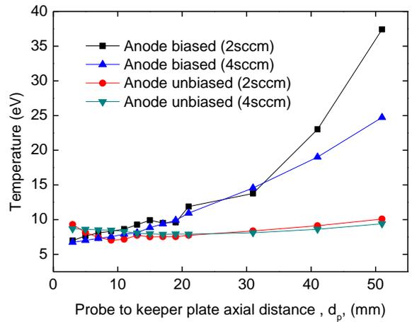
Figure 11. Electron temperature by Langmuir procedure
