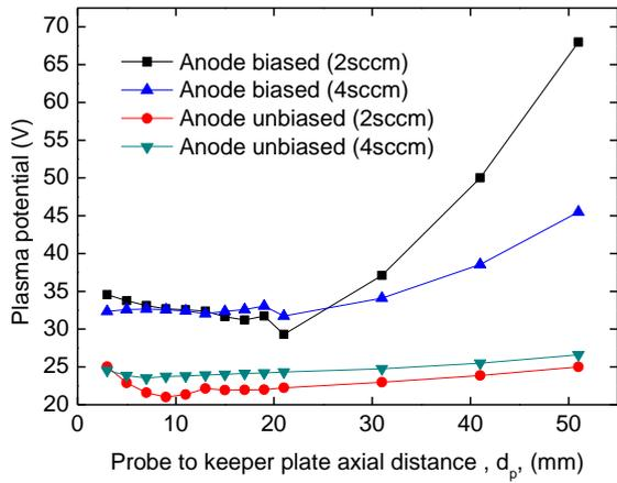
Figure 7. Plasma potential by Langmuir procedure
