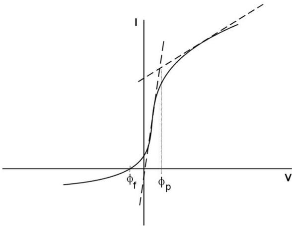
Figure 3. Typical I-V probe curves for cylindrical probe.
