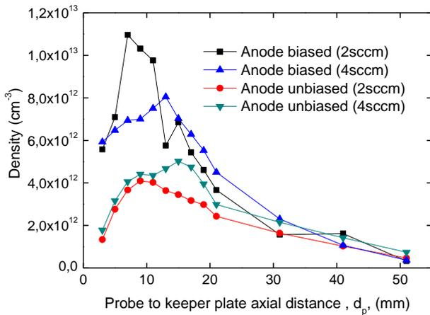
Figure 9. Mean electron density, Langmuir procedure
