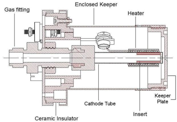
Figure 1. LAP hollow cathode schematics
