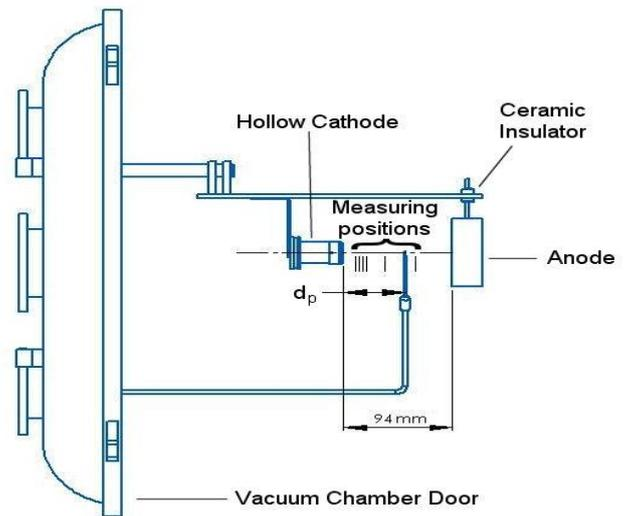
Figure 4. Hollow cathode assembled on the vacuum chamber door.  $d_p$ : distance from cylindrical probe to keeper.
