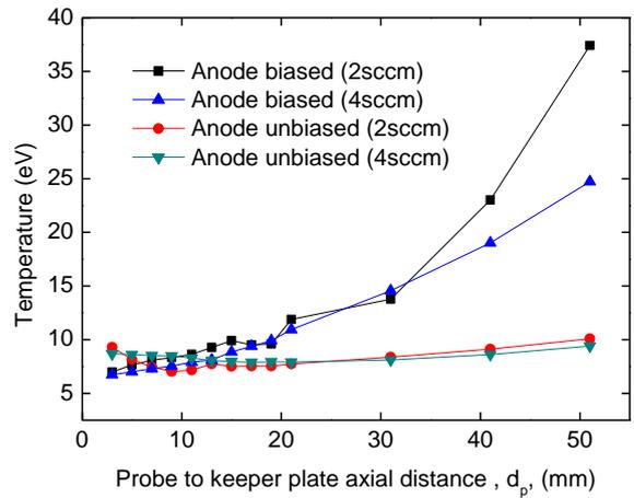
Figure 11. Electron temperature by Langmuir procedure
