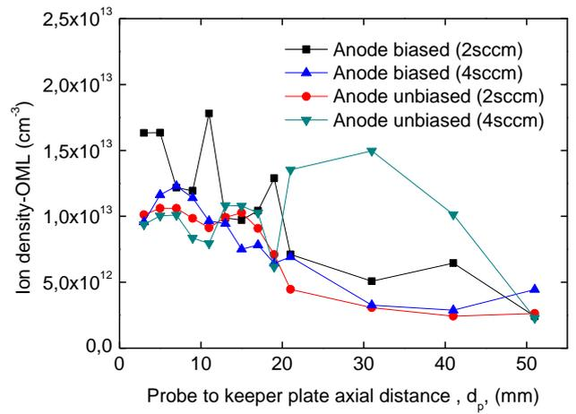
Figure 10. Ion density by orbital motion limited Theory, OML
