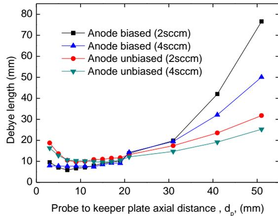
Figure 12. Debye length by Langmuir procedure
