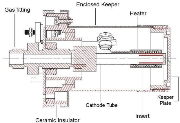
Figure 1. LAP hollow cathode schematics
