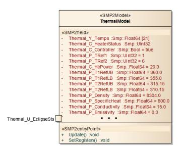
Figure 6.52 - SMP2 Thermal model responsible for handling the communication with the SINDA/FLUINT simulation.
