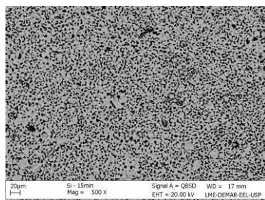
Figure 1 – SEM of porous silicon compact.
