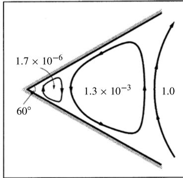
FIGURE 18. A drawing illustrating Moffatt eddies in a 60° concave corner. The values indicate the relative intensities (adapted from Moffatt (1964)).
