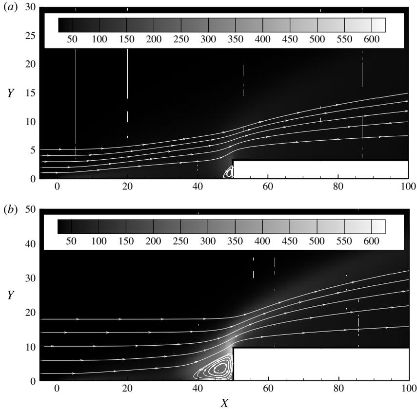
FIGURE 11. Contour maps for the pressure ratio ( $p/p_\infty$ ) for dimensionless frontal-face heights  $H$  of (a) 3.23 and (b) 9.69.
