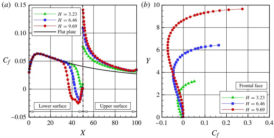
FIGURE 16. (Colour online) The distribution of the skin friction coefficient  $C_f$  along (a) the lower and upper surfaces and (b) the frontal-face surface parameterized by the dimensionless frontal-face height  $H$ .
