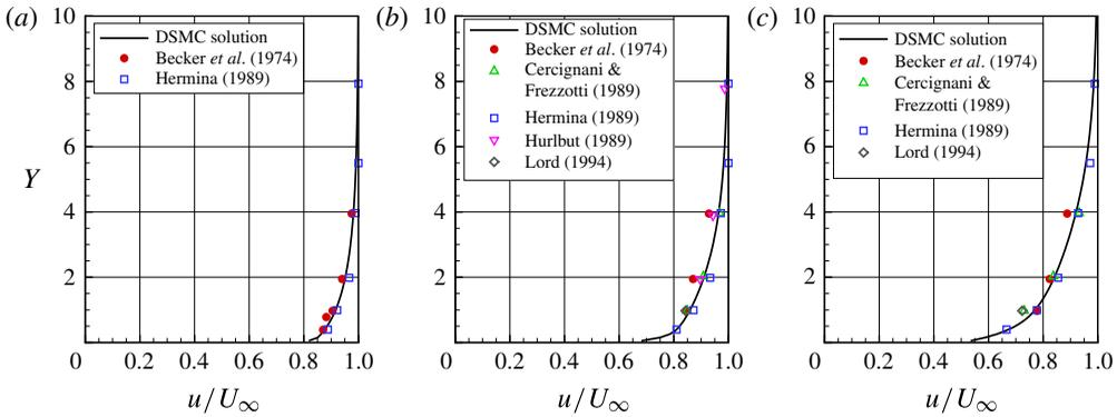
FIGURE 28. (Colour online) Tangential velocity ratio ( $u/U_\infty$ ) profiles normal to the flat-plate surface for three sections along the flat plate: (a)  $x=0.5$  mm, (b)  $x=2.5$  mm and (c)  $x=6.5$  mm. Solid lines represent the present DSMC simulations, full and empty symbols represent experimental and numerical data, respectively.
