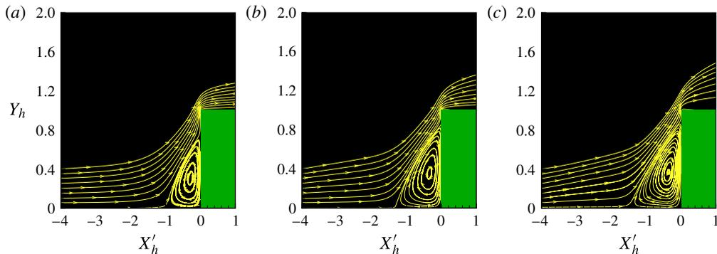
FIGURE 5. (Colour online) Distribution of streamline traces in the vicinity of the forward-facing step for dimensionless frontal-face heights  $H$  of (a) 3.23, (b) 6.46 and (c) 9.693.
