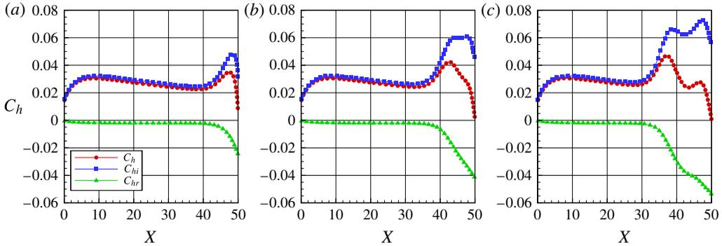
FIGURE 20. (Colour online) The distribution of the incident, reflected and total heat transfer coefficients along the lower surface of the step with height  $H$  of (a) 3.23, (b) 6.46, and (c) 9.69.
