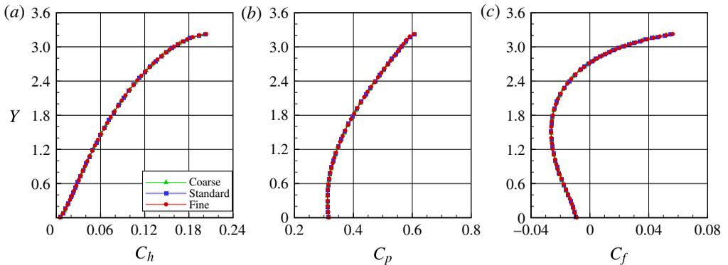
FIGURE 26. (Colour online) Effect of altering the cell size along the  $y$ -direction on (a) the heat transfer coefficient  $C_h$ , (b) the pressure coefficient  $C_p$  and (c) the skin friction coefficient  $C_f$  along the frontal-face surface for the  $H = 3.23$  case.
