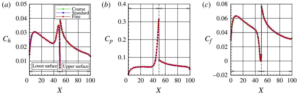
FIGURE 25. (Colour online) Effect of altering the cell size along the  $y$ -direction on (a) the heat transfer coefficient  $C_h$ , (b) the pressure coefficient  $C_p$  and (c) the skin friction coefficient  $C_f$  along the lower and upper surfaces for the  $H = 3.23$  case.
