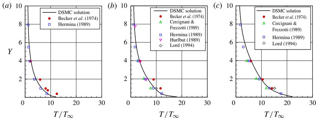
FIGURE 29. (Colour online) Temperature ratio ( $T/T_\infty$ ) profiles normal to the flat-plate surface for three sections along the flat plate: (a)  $x = 0.5$  mm, (b)  $x = 2.5$  mm and (c)  $x = 6.5$  mm. Solid lines represent the present DSMC simulations, full and empty symbols represent experimental and numerical data respectively.
