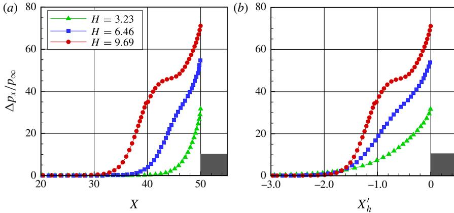
FIGURE 7. (Colour online) The upstream disturbance effect on the density due to the presence of the forward-facing step.
