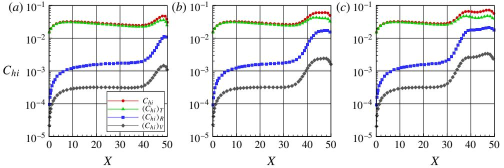
FIGURE 21. (Colour online) The contribution of translation, rotation and vibration energy modes to the incident heat transfer coefficient along the lower surface of the step with height  $H$  of (a) 3.23, (b) 6.46 and (c) 9.69.
