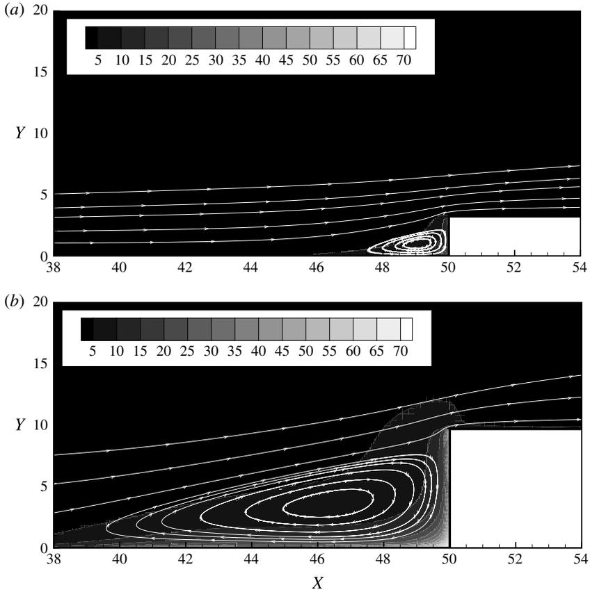
FIGURE 8. Contour maps for the density ratio ( $\rho/\rho_\infty$ ) for dimensionless frontal-face heights  $H$  of (a) 3.23 and (b) 9.69.
