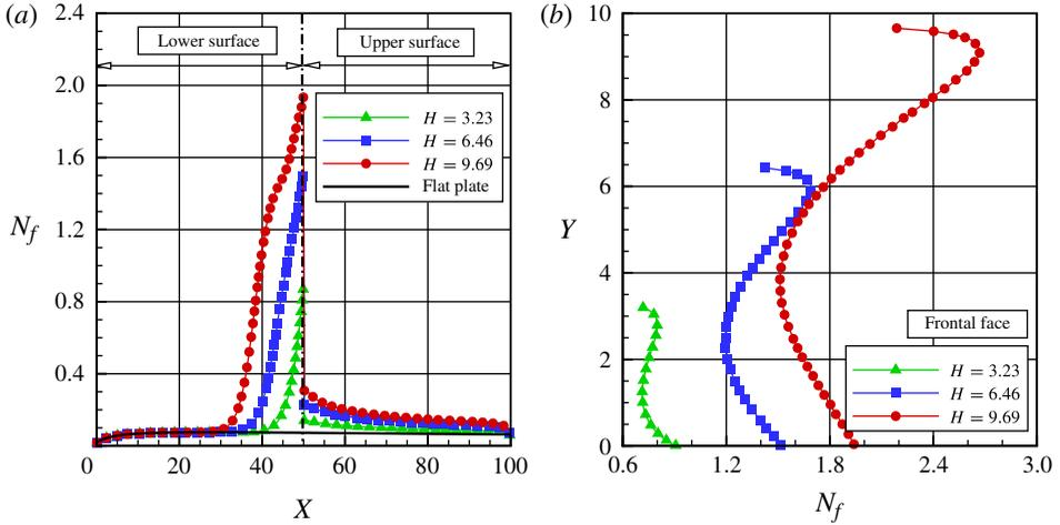
FIGURE 14. (Colour online) The distribution of the number flux  $N_f$  along (a) the lower and upper surfaces and (b) the frontal-face surface parameterized by the dimensionless frontal-face height  $H$ .
