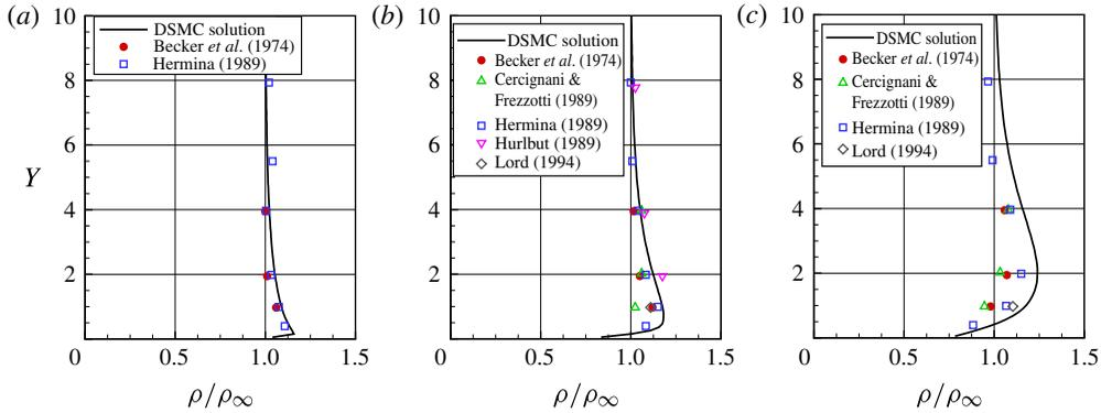
FIGURE 27. (Colour online) Density ratio ( $\rho/\rho_\infty$ ) profiles normal to the flat-plate surface for three sections along the flat plate: (a)  $x=0.5$  mm, (b)  $x=2.5$  mm and (c)  $x=6.5$  mm. Solid lines represent the present DSMC simulations, full and empty symbols represent experimental and numerical data respectively.
