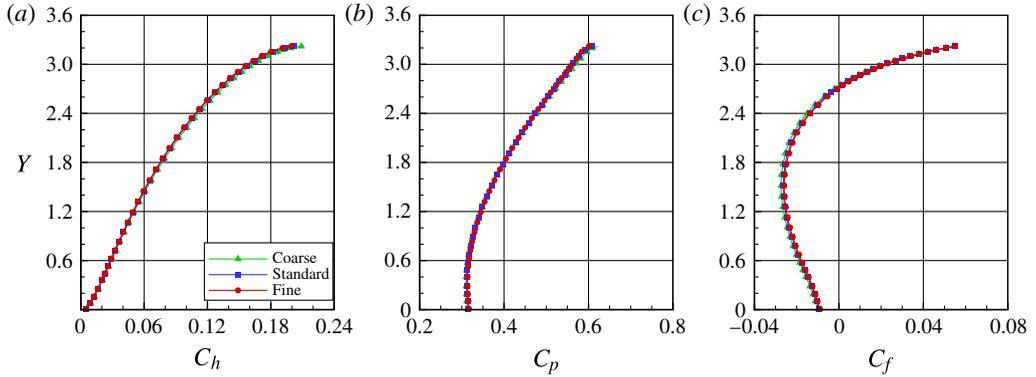
FIGURE 24. (Colour online) Effect of altering the cell size along the  $x$ -direction on (a) the heat transfer coefficient  $C_h$ , (b) the pressure coefficient  $C_p$  and (c) the skin friction coefficient  $C_f$  along the frontal-face surface for the  $H = 3.23$  case.
