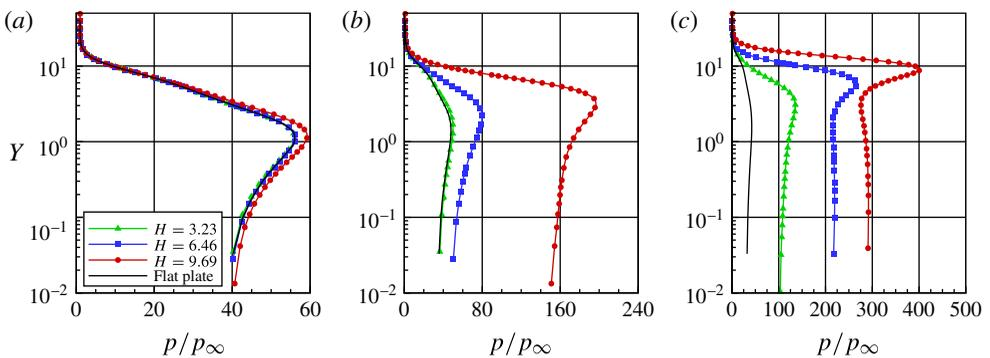
FIGURE 9. (Colour online) Pressure ratio ( $p/p_\infty$ ) profiles for a section  $X$  of (a) 28, (b) 38 and (c) 48 along the lower surface of the forward-facing step parameterized by the dimensionless frontal-face height  $H$ .
