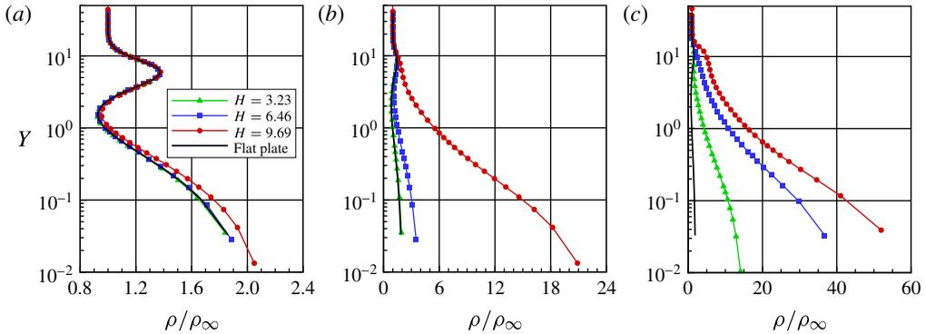
FIGURE 6. (Colour online) Density ratio ( $\rho/\rho_\infty$ ) profiles for a section  $X$  of (a) 28, (b) 38 and (c) 48 along the lower surface of the forward-facing step parameterized by the dimensionless frontal-face height  $H$ .
