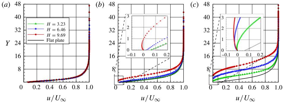
FIGURE 4. (Colour online) Tangential velocity ratio ( $u/U_\infty$ ) profiles for a section  $X$  of (a) 28, (b) 38 and (c) 48 along the lower surface of the forward-facing step parameterized by the dimensionless frontal-face height  $H$ .
