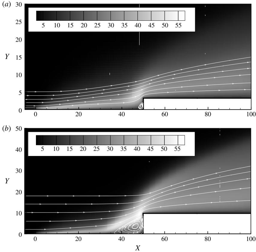
FIGURE 13. Contour maps for the overall temperature ratio ( $T_0/T_\infty$ ) for dimensionless frontal-face heights  $H$  of (a) 3.23 and (b) 9.69.
