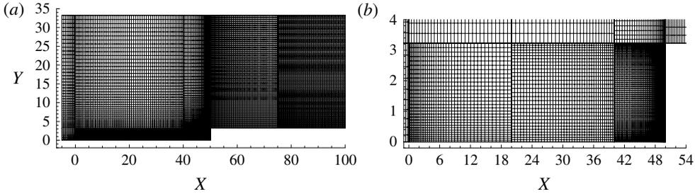
FIGURE 3. A drawing illustrating the cell distribution for (a) the standard grid for the  $H=3.23$  case and (b) a magnified view of regions R2, R3 and R4 in the vicinity of the step frontal face.
