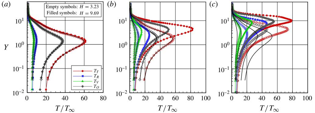
FIGURE 12. (Colour online) Kinetic temperature ratio ( $T/T_\infty$ ) profiles for a section  $X$  of (a) 28, (b) 38 and (c) 48 along the lower surface of the forward-facing step parameterized by the dimensionless frontal-face height  $H$ .
