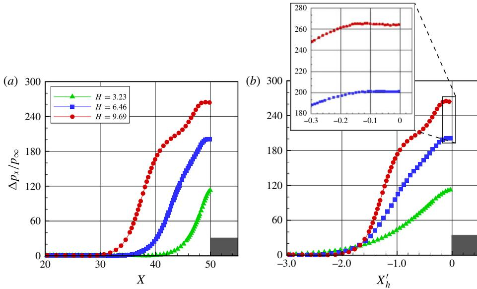
FIGURE 10. (Colour online) The upstream disturbance effect on pressure due to the presence of the forward-facing step.
