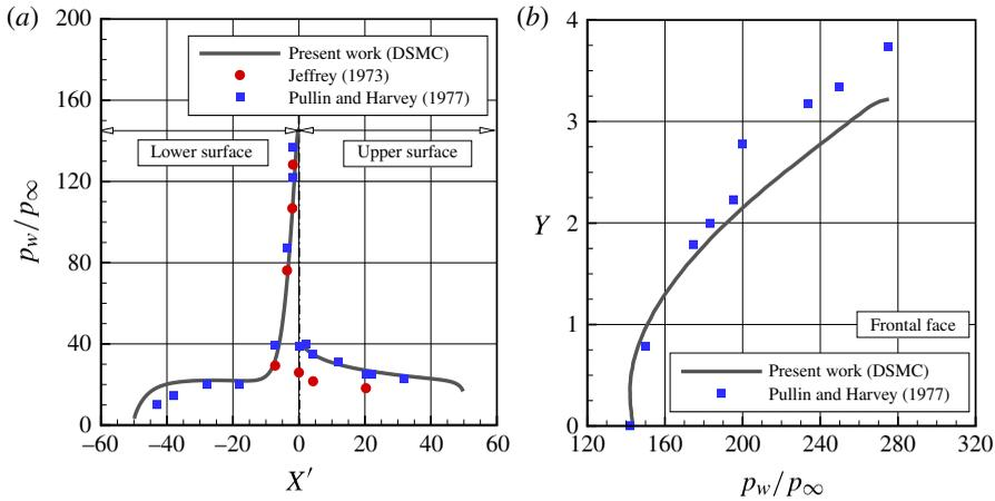
FIGURE 22. (Colour online) Comparison of the pressure ratio ( $p_w/p_\infty$ ) distribution acting along (a) the lower and upper surfaces and (b) the frontal-face surface for the  $H = 3.23$  case.
