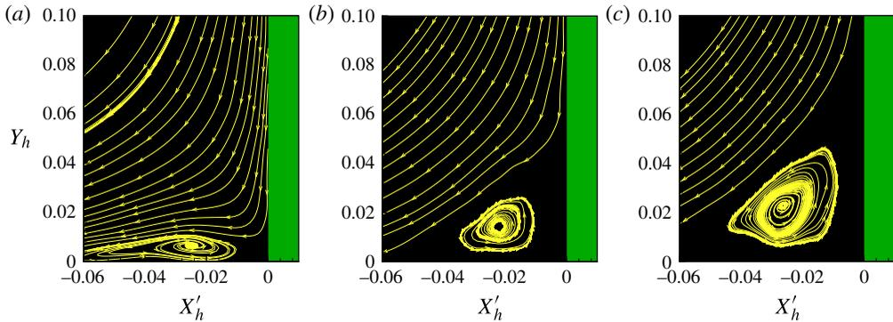
FIGURE 17. (Colour online) The distribution of the streamline traces in the vicinity of the step base for dimensionless frontal-face heights  $H$  of (a) 3.23, (b) 6.46 and (c) 9.69.
