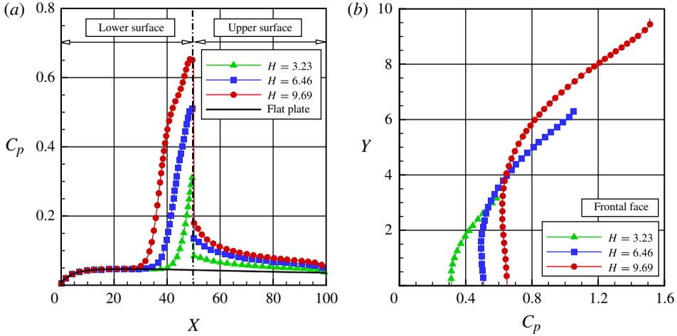
FIGURE 15. (Colour online) The distribution of the pressure coefficient  $C_p$  along (a) the lower and upper surfaces and (b) the frontal-face surface parameterized by the dimensionless frontal-face height  $H$ .
