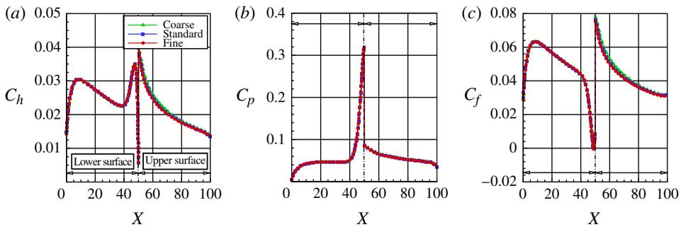
FIGURE 23. (Colour online) Effect of altering the cell size along the *x*-direction on (a) the heat transfer coefficient  $C_h$ , (b) the pressure coefficient  $C_p$  and (c) the skin friction coefficient  $C_f$  along the lower and upper surfaces for the  $H = 3.23$  case.
