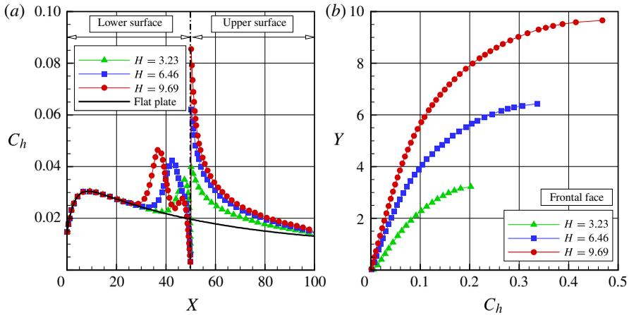
FIGURE 19. (Colour online) The distribution of the heat transfer coefficient  $C_h$  along (a) the lower and upper surfaces and (b) the frontal-face surface parameterized by the dimensionless frontal-face height  $H$ .
