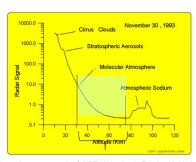
The figure shows an example of INPE's Lidar signal. The signal is blocked from 0 to 12 km. Cirrus clouds and stratospheric aerosols overlap the atmospheric molecular signal from 15 to 30 km. Resonant scattering of sodium are obtained from 78 to 105 km. From 30 to 75 km clean molecular Rayleigh signal is used to measure the atmospheric density and temperature.
