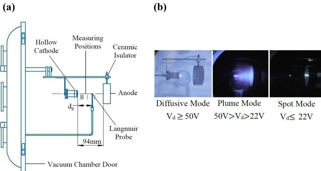
Figure 1. Experimental setup (a) and discharge modes of hollow cathodes (b).
