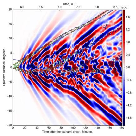
Figure 4. Simulated traveltime diagram (TTD) for the realistic Case II. This TTD is constructed by time scanning the  $\Delta$ TEC along a chosen horizontal trajectory which is shown as a blue line in Fig. 3. The background image represents the  $\Delta$ TEC disturbance or TIDs and the green-blue contours represent contours of the main, simulated, tsunami waves.
