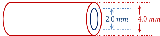
Figure A.1. Dimensions of the coaxial line used by Weiner.
