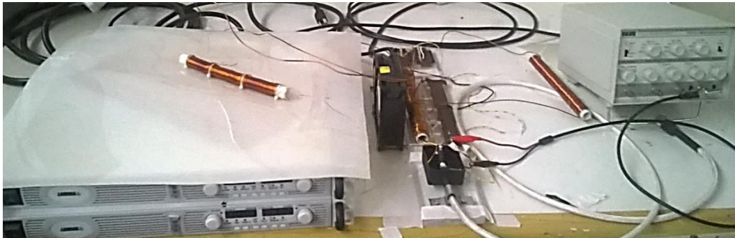
Figure 5.28. Experimental assembly with axial and azimuthal bias for low voltage operation.
