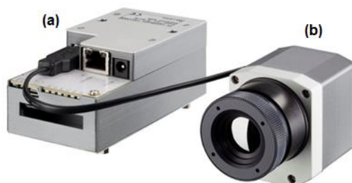
Figura 3.1 - Kit Optris PI LightWeight (a) Microprocessador e (b) Sensor IV termal Optris PI450 LW.
