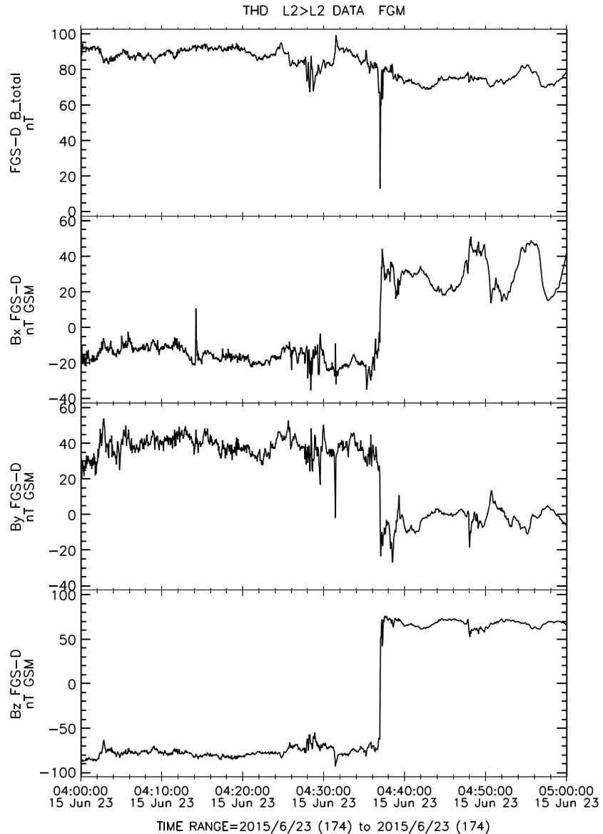
**Figure 4.** Magnetic field data from THEMIS D on 23 June 2015. The crossing of the magnetopause is evident around 0437 UT.
