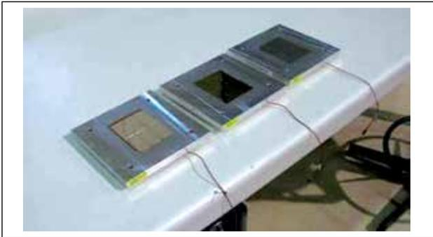
Figure 3. OSR coupons used in the environmental tests.
