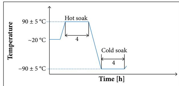
**Figure 9.** Theoretical curve for test in thermal-vacuum chamber.
