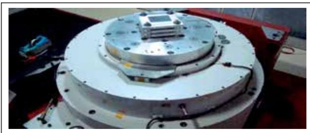
**Figure 7.** Set of coupons installed for vibration testing.
