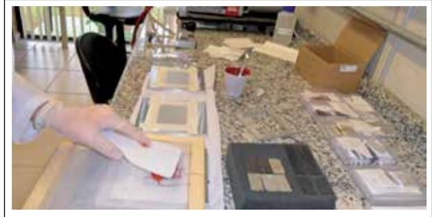
Figure 6. Printing screen being used to apply the RTV566 on aluminum plates.
