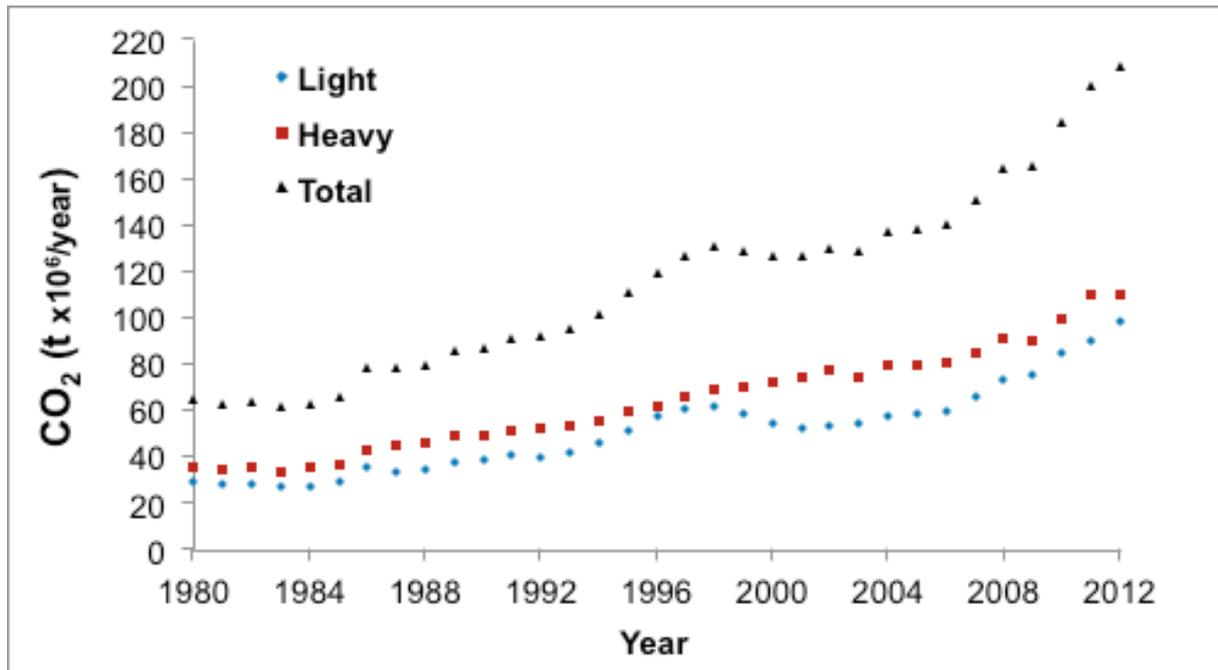
Figure 4 – Absolute CO<sub>2</sub> emissions for Otto and Diesel cycles vehicles.
