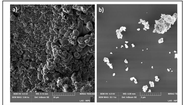
**Figure 2: Field Emission Scanning Electron Microscopy (SEM-FEG) (a) Diamond (b) after 3 hours of MAE.**
