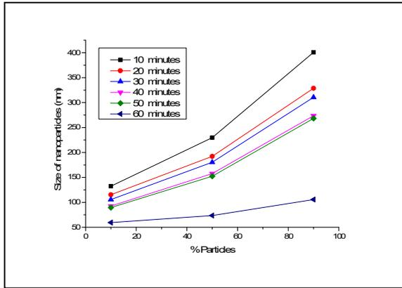
**Figure 1: Effect of centrifugation time on particle size (D90).**
