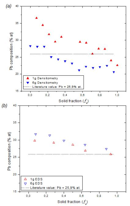
**Fig. 3.** Lead composition profile for 1g and 6g PbSn eutectic alloy analyzed by densitometry (a); energy dispersive spectrometry (EDS) (b).
