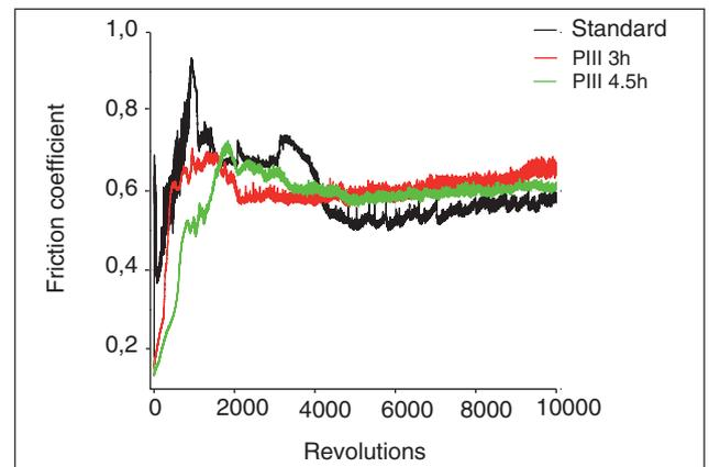
Figure 7: Friction coefficient curves of the SS304 alloys.
