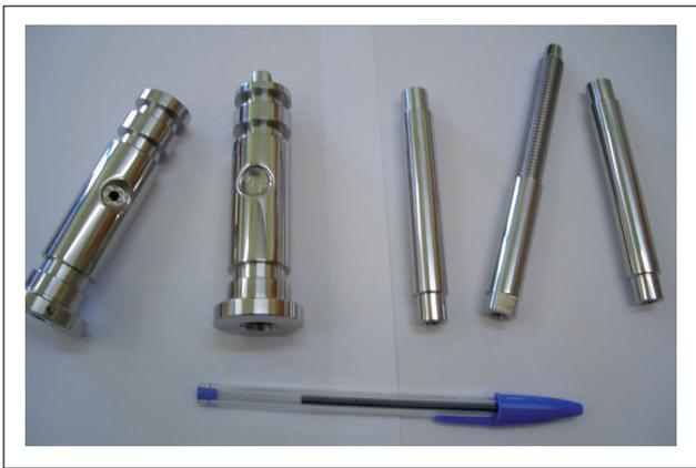
**Figure 9:** Camera components treated by PIII.
