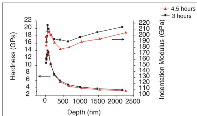
Figure 6: Hardness and indentation modulus profiles of PIII treated SS304.
