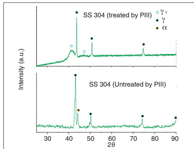
Figure 2: X-ray diffractograms of treated and untreated SS304.
