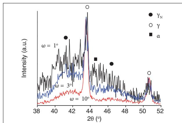
Figure 3: Glancing incidence X-ray diffractograms of treated SS304.
