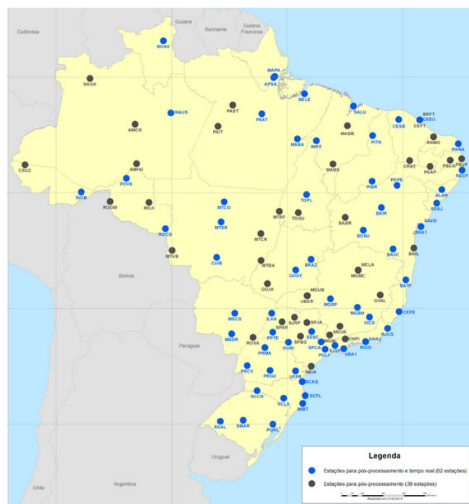
Figure 4. Stations configuration of RBMC. Blue points: real time stations; black points: post-processed stations. Image from IBGE website, available at < http://www.ibge.gov.br/home/geociencias/geodesia/rbmc/rbmc_est.php >.
