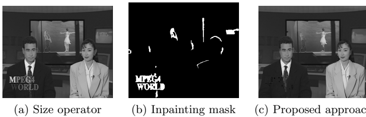
Figure 5. Example of filtering with the size criterion.
