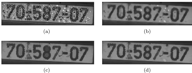
Figure 4. (a) Input image, artificially corrupted, (b) filtered with a median filter, (c) filtered with regular self dual opening by reconstruction, and (d) filtered by the EWT-based opening by reconstruction, using circle SE of radius 4.
