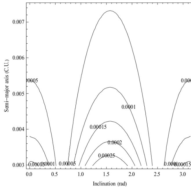
**Figure 8.**  $PI_3$  as a function of the semi-major axis (in canonical units) and inclination (in radians) for eccentric orbits for spacecraft considering the effects of the irregular shape of Europa.
