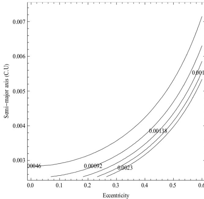
**Figure 10.**  $PI_1$  as a function of the semi-major axis (in canonical units) and eccentricity for eccentric orbits for spacecraft considering the effects of the irregular shape of Europa.
