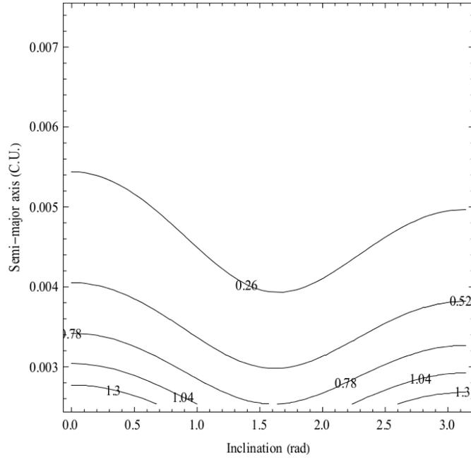
**Figure 3.**  $PI_1$  as a function of the semi-major axis (in canonical units) and inclination (in radians) of circular orbits for the spacecraft considering only the third-body effects of Jupiter and the terms coming from the rotating frame.
