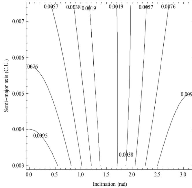
**Figure 9.**  $PI_3$  as a function of the semi-major axis (in canonical units) and inclination (in radians) for eccentric orbits for spacecraft considering the effects of the third-body perturbation from Jupiter and the effects of the rotating frame.
