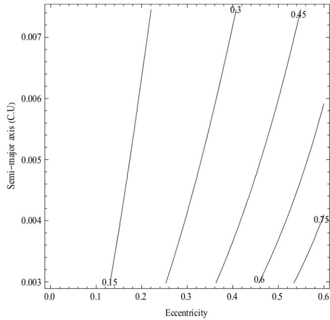
Figure 12.  $PI_3$  as a function of the semi-major axis (in canonical units) and eccentricity for eccentric orbits for spacecraft considering the effects of the irregular shape of Europa, the third-body perturbation from Jupiter and the effects of the rotating frame.
