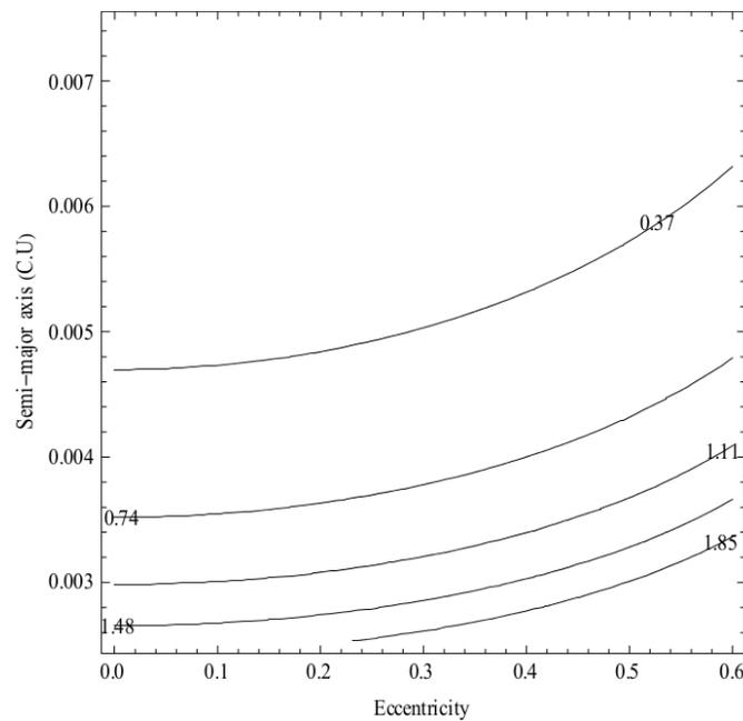
**Figure 11.  $PI_1$  as a function of the semi-major axis (in canonical units) and eccentricity for eccentric orbits for spacecraft considering the effects of the irregular shape of Europa, the third-body perturbation from Jupiter and the effects of rotating frame.**
