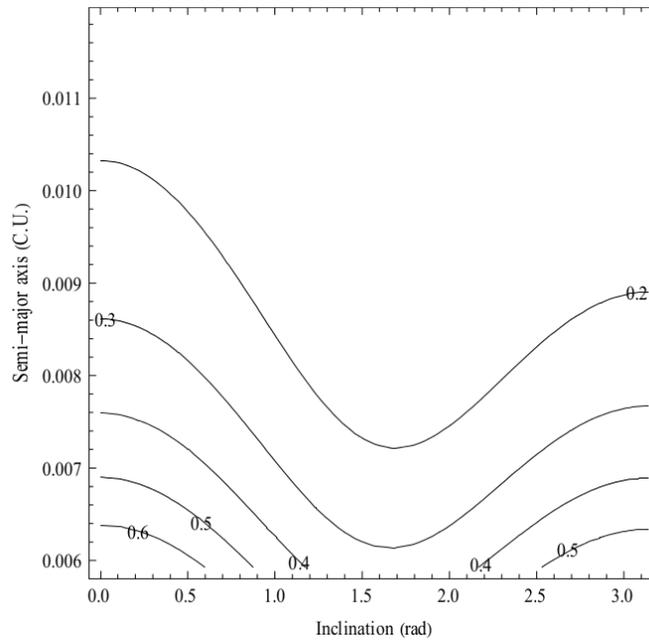
**Figure 19.**  $PI_1$  as a function of the semi-major axis (in canonical units) and eccentricity for eccentric orbits for spacecraft considering the effects of the irregular shape of Callisto, the third-body perturbation from Jupiter and the effects of the rotating frame.
