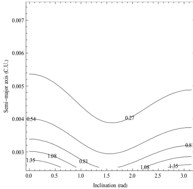
**Figure 4.**  $PI_1$  as a function of the semi-major axis (in canonical units) and inclination (in radians) of circular orbits for the spacecraft considering the third-body effects of Jupiter, the terms coming from the rotating frame and the irregular shape of Europa.
