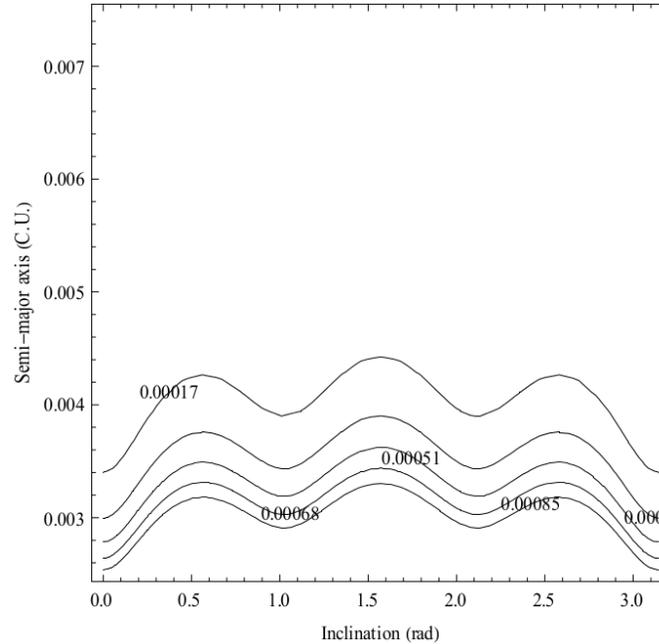
**Figure 2.**  $PI_1$  as a function of the semi-major axis (in canonical units) and inclination (in radians) of circular orbits for the spacecraft considering only the effects of the irregular shape of Europa.
