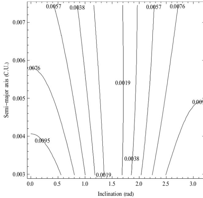
**Figure 7.**  $PI_3$  as a function of the semi-major axis (in canonical units) and inclination (in radians) for eccentric orbits for spacecraft considering the third-body effects of Jupiter, the irregular shape of Europa and the terms due to the rotating frame.
