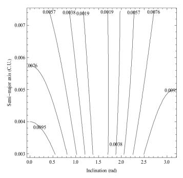
Figure 9.  $PI_3$  as a function of the semi-major axis (in canonical units) and inclination (in radians) for eccentric orbits for spacecraft considering the effects of the third-body perturbation from Jupiter and the effects of the rotating frame.
