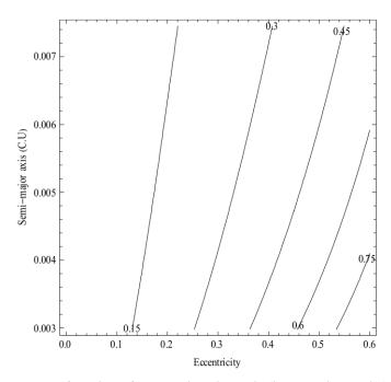
Figure 12.  $PI_3$  as a function of the semi-major axis (in canonical units) and eccentricity for eccentric orbits for spacecraft considering the effects of the irregular shape of Europa, the third-body perturbation from Jupiter and the effects of the rotating frame.
