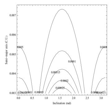
Figure 8.  $PI_3$  as a function of the semi-major axis (in canonical units) and inclination (in radians) for eccentric orbits for spacecraft considering the effects of the irregular shape of Europa.
