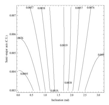
Figure 7.  $PI_3$  as a function of the semi-major axis (in canonical units) and inclination (in radians) for eccentric orbits for spacecraft considering the third-body effects of Jupiter, the irregular shape of Europa and the terms due to the rotating frame.
