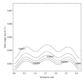
Figure 2.  $PI_1$  as a function of the semi-major axis (in canonical units) and inclination (in radians) of circular orbits for the spacecraft considering only the effects of the irregular shape of Europa.
