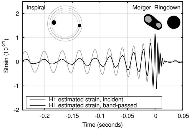
**FIG. 1. Simulated waveform:** Predicted strain in H1 for a source with parameters  $q = 1.22$ ,  $\chi_{1,z} = 0.33$ ,  $\chi_{2,z} = 0.44$ , simulated in full general relativity; compare to Figure 2 in LVC-detect[2]. The gray line shows the idealized strain response  $h(t) = F_+h_+(t) + F_xh_x(t)$ , while the solid black line shows the whitened strain response, using the same noise power spectrum as LVC-detect[2].
