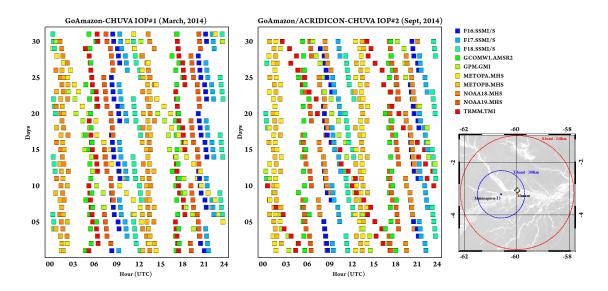
Overpasses within a 60 km radius of the X-band CHUVA radar (on right). SOURCE: Author's production.
