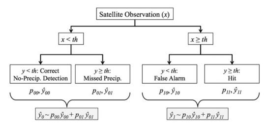
Figure 2.3 - Schematic of the PUSH satellite precipitation error scheme.
