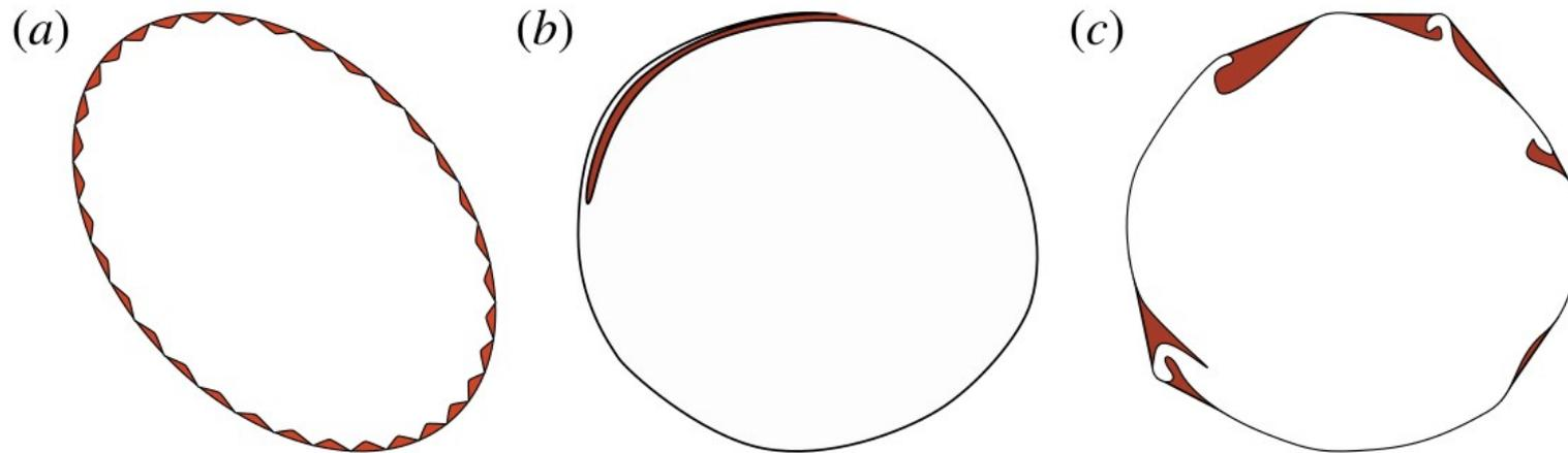
The outer line defines the convex-hull, the smallest convex set that contains the inner set.
