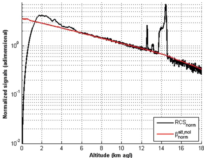
**FIG. 6.** Example of Rayleigh fit for the channel 532 photon-counting mode for system SPU (São Paulo, Brazil) on 17 Sep 2015. Molecular signal (in red) represents the theoretical behavior expected under clean conditions (no aerosol particles or clouds). The measured lidar signals, normalized at the height range 10–12 km, are shown in black.
