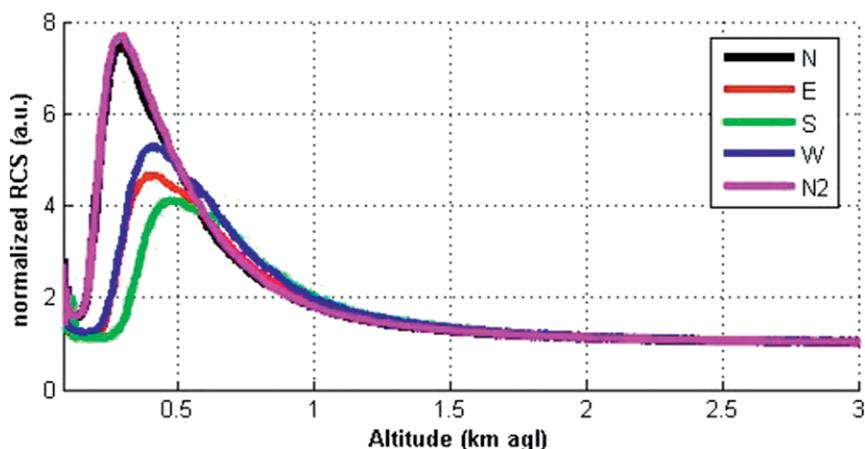
**FIG. 5.** Example of quadrant telecover test of the channel 355 analog mode for system MAO (Manaus, Brazil) on 9 Jun 2015. Colors refer to the different quadrants: North (N, black), East (E, red), South (S, green), West (W, blue), and North2 (N2, magenta). Curves represent the lidar RCS normalized at the height range 4–5 km.
