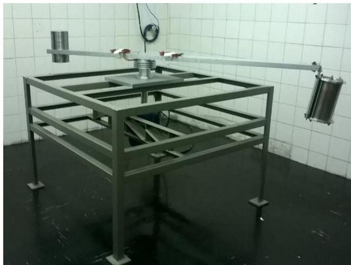
**Fig. 1.** Centrifuge (with furnace at the right side) of LAS/INPE.
