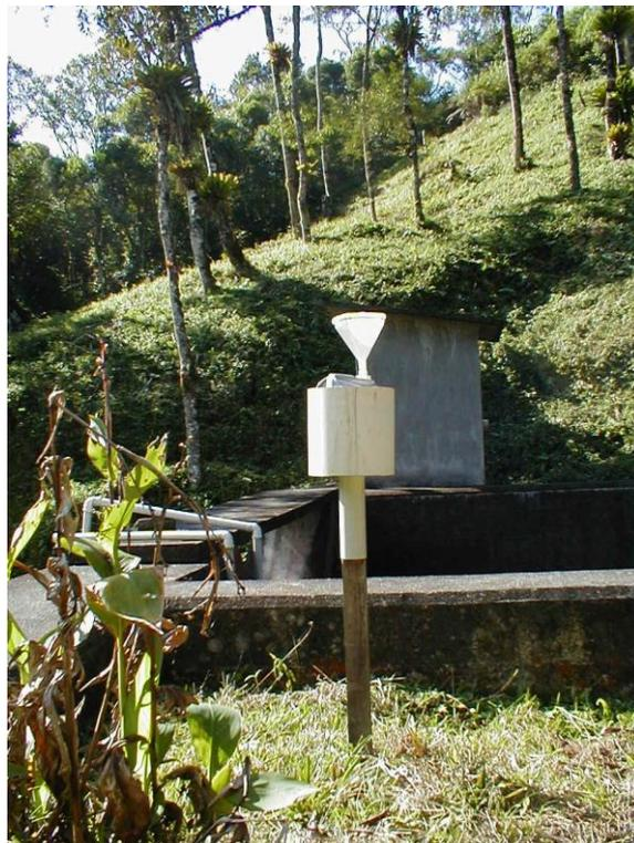
Figure 1a – Picture of the bulk collector installed next to the catchment B weir at CUNHA (Forti, 2000).
