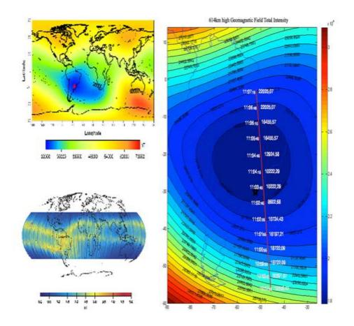
Figure 5: The South America Magnetic Anomaly - SAMA region Geomagnetic Field total Intensity (top left) and Equatorial Electron Jet - EEJ (bottom left) - Ref<sup>3,4</sup>. Results from NANOSATC-BR1 Scientific Mission Payload measurements of the SAMA region (right).
