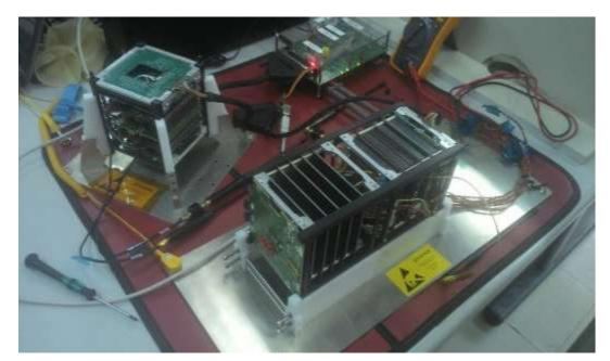
Figure 1: The NANOSATC-BR1 and NANOSATC-BR2 Engineering Model Platforms.
