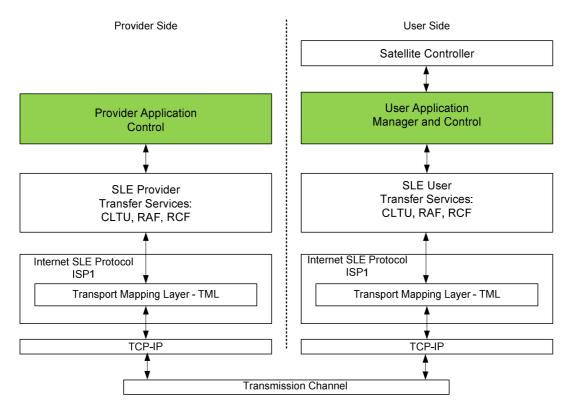
Figure 8. Architecture Model based on ISP1
