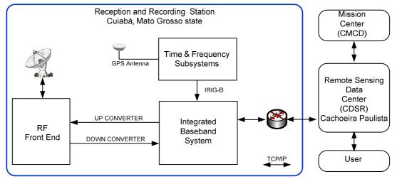
Figure 3. X-Band Reception and Recording Station
