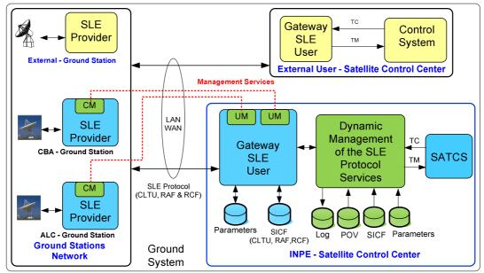
Figure 9. Environment for satellite operation with the dynamic management of the SLE protocol services
