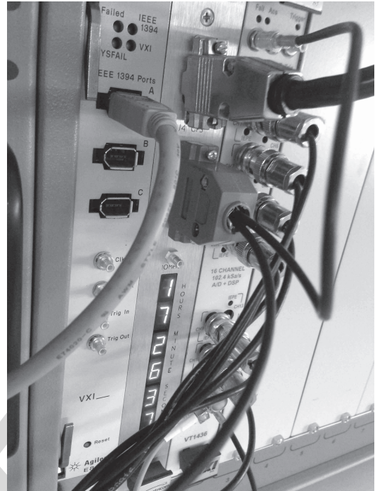
Fig. 6. Picture showing the three boards. BC537gps is located in the middle where one can see the 15 pin D plug with two cables (PPS and the external clock signals) leaving it. Just above it, the cable to the GPS antenna can be seen. VT1436 board is on the right and the E8491B board is on the left.
