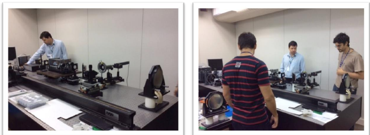
Figure 28: The images show team members working on the alignment of the Fabry-Perot Etalon.
