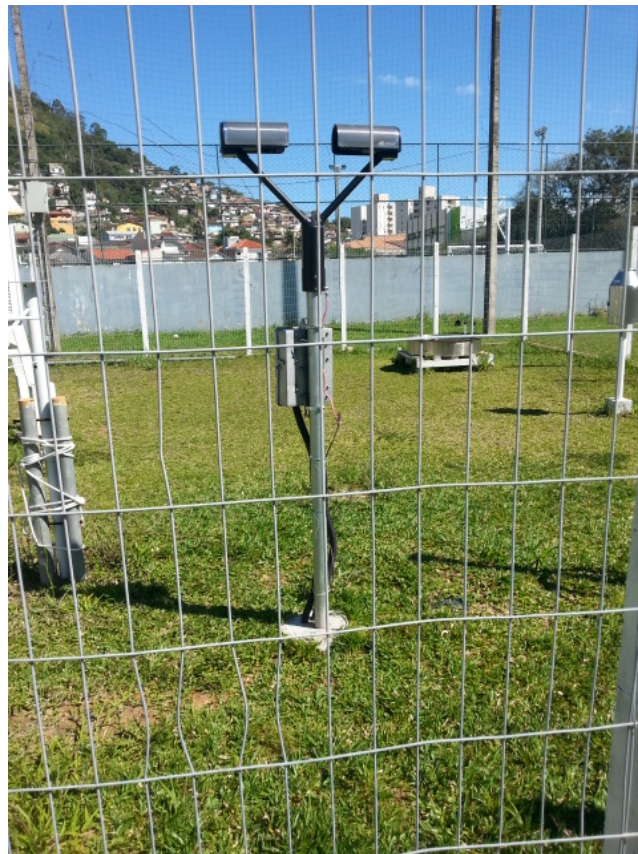
Figure 1.1 - PARSIVEL 2 site overview.
