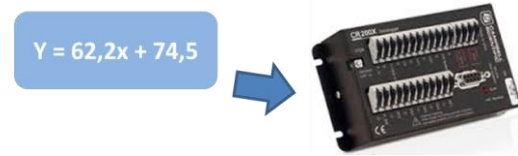
Figure 4. Offset adjustment and multiplier factor applied to a datalogger used in a weather station
