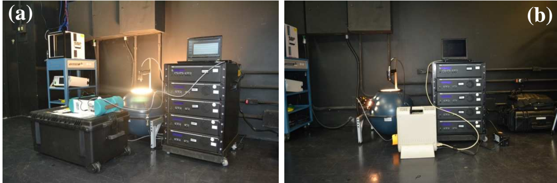
Figure 3.8. Overview of the experimental setup to characterize and assess the spectroradiometer. In (a) the FieldSpec Pro ASD used in fieldwork; and (b) the FieldSpec Pro ASD belonging to the LaRaC laboratory, which remains all the time in the laboratory, therefore, is an instrument considered as a reference.
